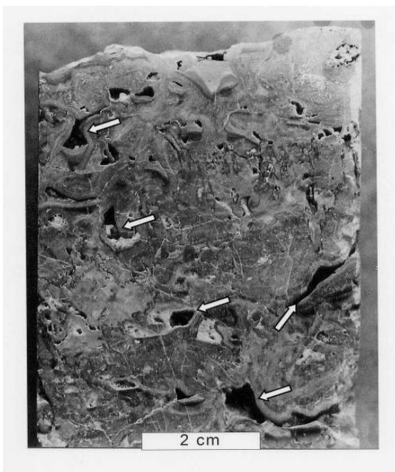
Figure 4. Core slab with secondary vugs (arrows) resulting from the partial dissolution of earlier dolomite cement (white).
